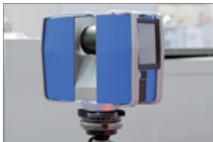
Laser scanner for 3D metrology
