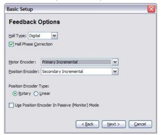
The CME2 screen above shows a Primary Incremental encoder for the motor input. Other types of encoders can be selected for this function. The secondary encoder input can be used for either motor or position feedback.
