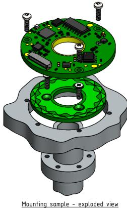
Note: While using an encoder rotor adaptor (which isn't part of the motor shaft), the adaptor should be made from a nonmetal material.
